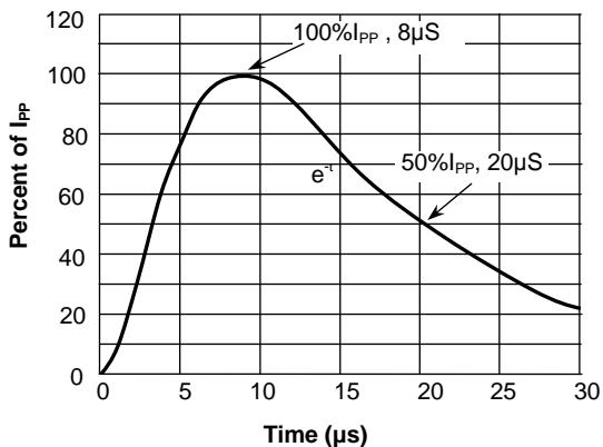
**Fig.4 Pulse Waveform-ESD(IEC61000-4-2)**
